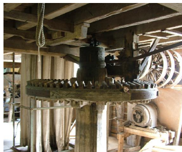
ALDERFORD WATER MILL; Nick Joscelyne presenting the apple log to Brian Mills, with pictures of the cog wheel where the wooden teeth are located.
